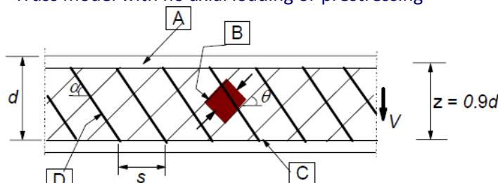
[A] - compression chord, [B] - struts, [C] - tensile chord, [D] - shear reinforcement
